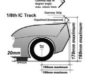
Am, GT1 and GT2 cars max. width: 267 mm max. height: 170 mm (on 20 mm blocs) Overall, maximum height including a Gurney strip 180 mm (on 20 mm blocs) max distance behind rear axle: 100 mm (110 mm for 2wd & flat chassis cars).
